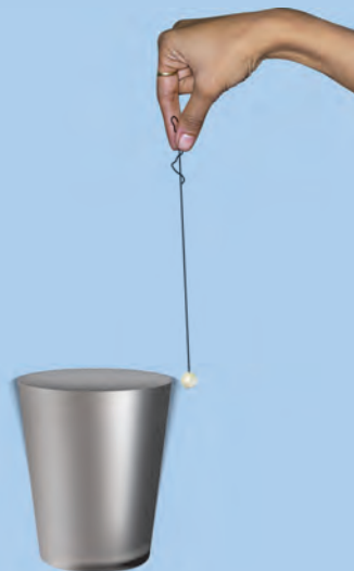
Fig. 13.17 : Thermocol ball touching the vibrating glass tumbler
